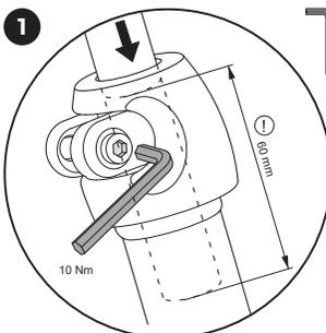
Insert the handlebar into the steer tube and tighten the screw. Please pay attention to the marking of the minimum insertion depth.
