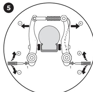
Now centre the brake arms by turning the adjusting screw. You will need a crosslip screwdriver for this.
