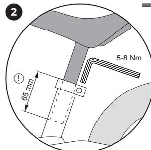
After loosening the saddle clamp, you can pull out the saddle (observe minimum insertion depth). Then retighten (5-8 Nm). The brake on this bike has already been installed and adjusted by PUKY.
