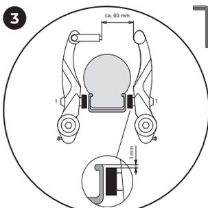
**Settings control and fine adjustment of the brake (V-brake).**
